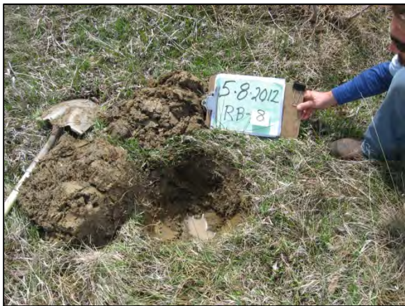
May 8, 2012. Sample point RB-8. Close up of groundwater observation hole.
