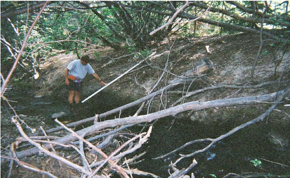
Figure 5-3. Bank undercutting to a depth of 5ft on Third Creek (station 12+00).
