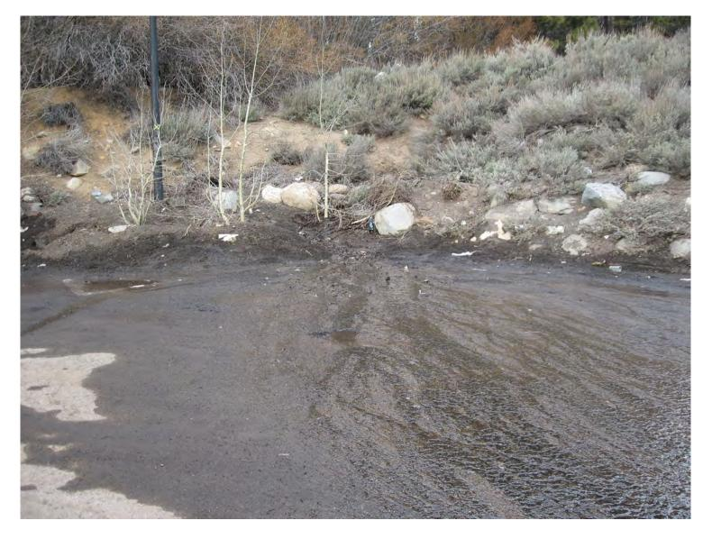
As a result of a 1980 restoration project, Burke Creek runs along a knoll. Consequently the stream escapes its channel in numerous spots because of its perched location. Some of the escaped stream flows across the Lam Watah trail and into the trailhead parking lot. This escaped flow signifies instability as the stream finds a new channel and could result in a new stream channel in an undesirable location.
