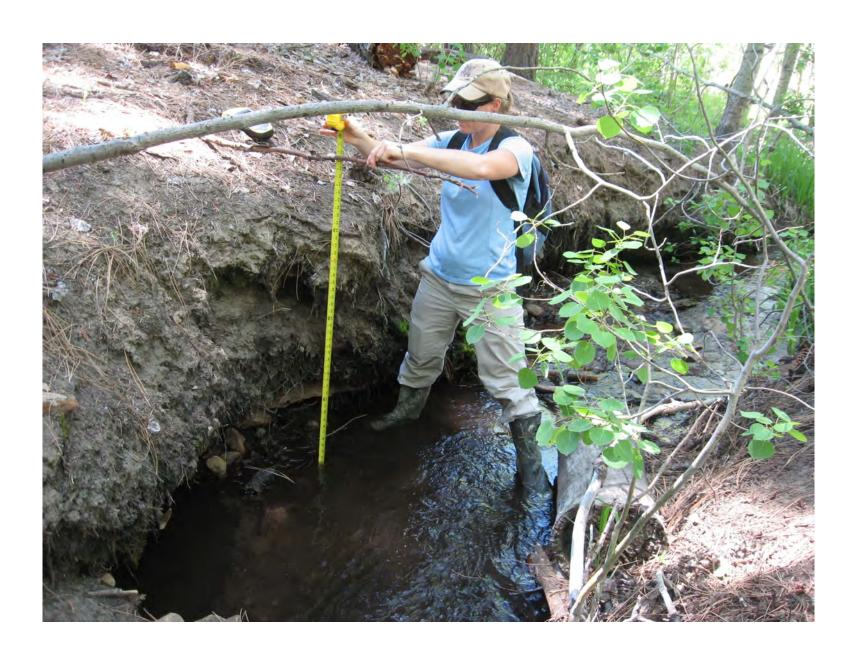
Head cuts are causing channel entrenchment, bank undercutting and erosion.
