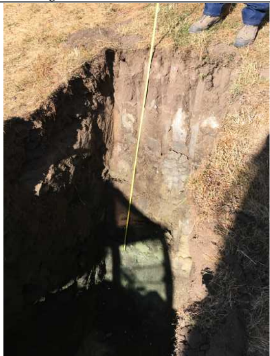
Test Pit no. 2 – Depth of fill material is about 6 feet. Mixed rock and soil fill. Groundwater at 4.5 feet.
