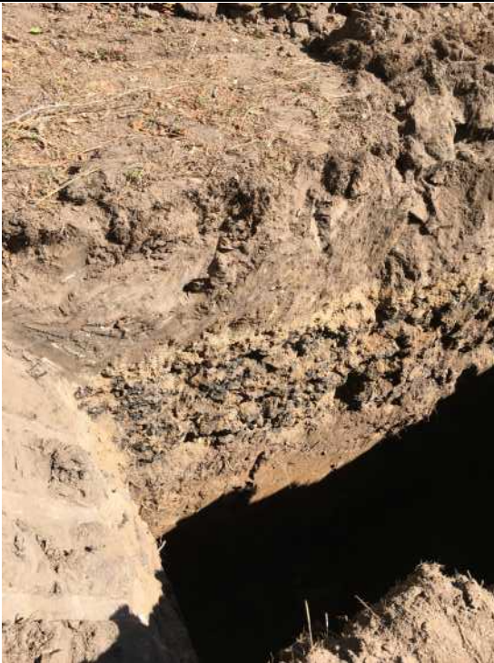
Test Pit no. 4 – Dug to 14 feet, but native soil at 8 feet. Groundwater observed at 10 feet (higher in spring).
