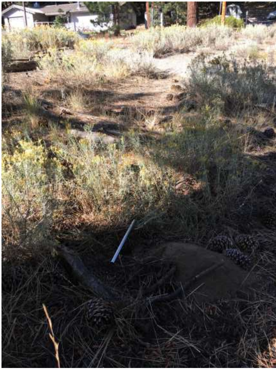
Auger Hole 1 – Hand augered to 55+in. depth. No evidence of water table or restricting layer.
