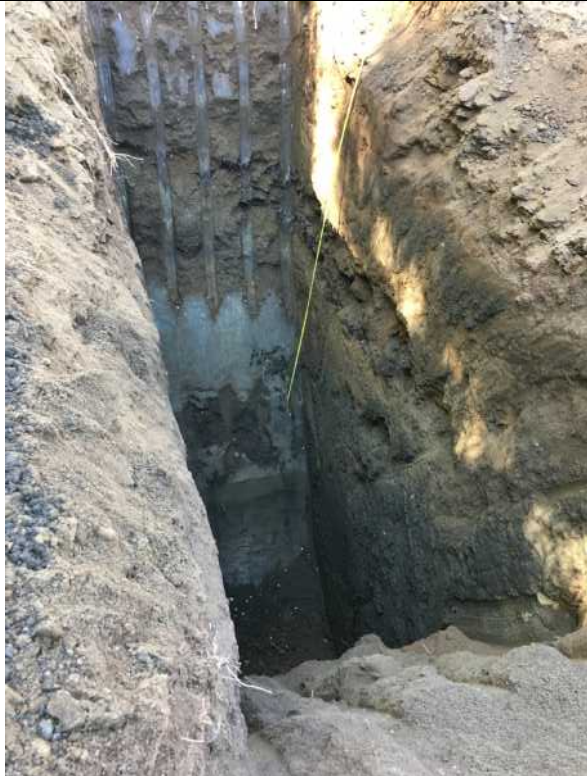
Test Pit no. 3 – Dug to 12 feet, but native soil at 7.5 feet. Groundwater not observed (naturally dry in fall).
