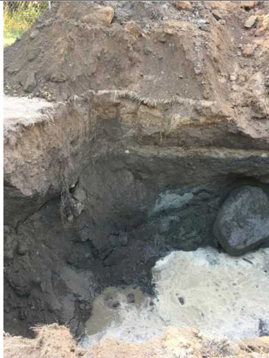
Test Pit no 1 – Multiple layers of fill material in upper 4.5 ft. Gray soil at 3+ feet infers high water table.
