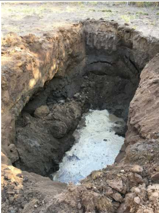
Test Pit no. 1 – Dug to 10 ft. Water poured in from surrounding fill material, so native soil not observed.
