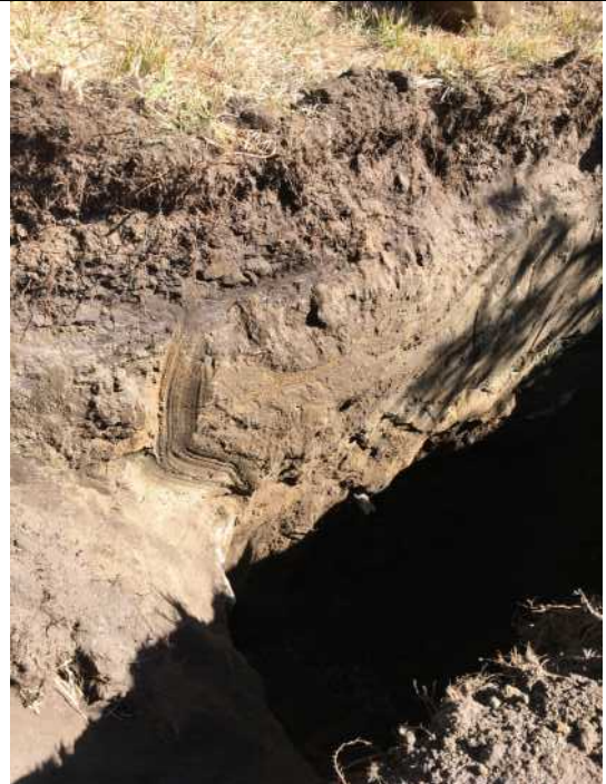
Test Pit no. 5 – Depth of fill material is 8.5 feet, then native soil. Groundwater at 9 feet (higher in spring).
