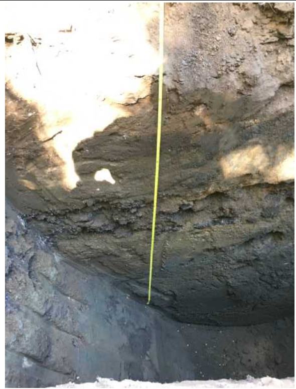
Test Pit no 3 – Fill material has a 1-ft. thick layer of soil and crushed asphalt at 4-foot depth.
