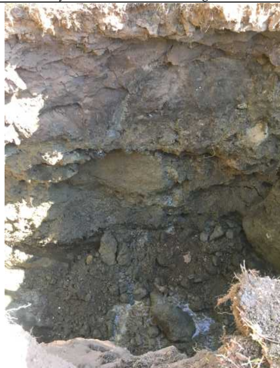
Test Pit no 2 – Fill material is mostly fines in upper 2 feet, then increased gravels, cobbles and stones to 6 feet.
