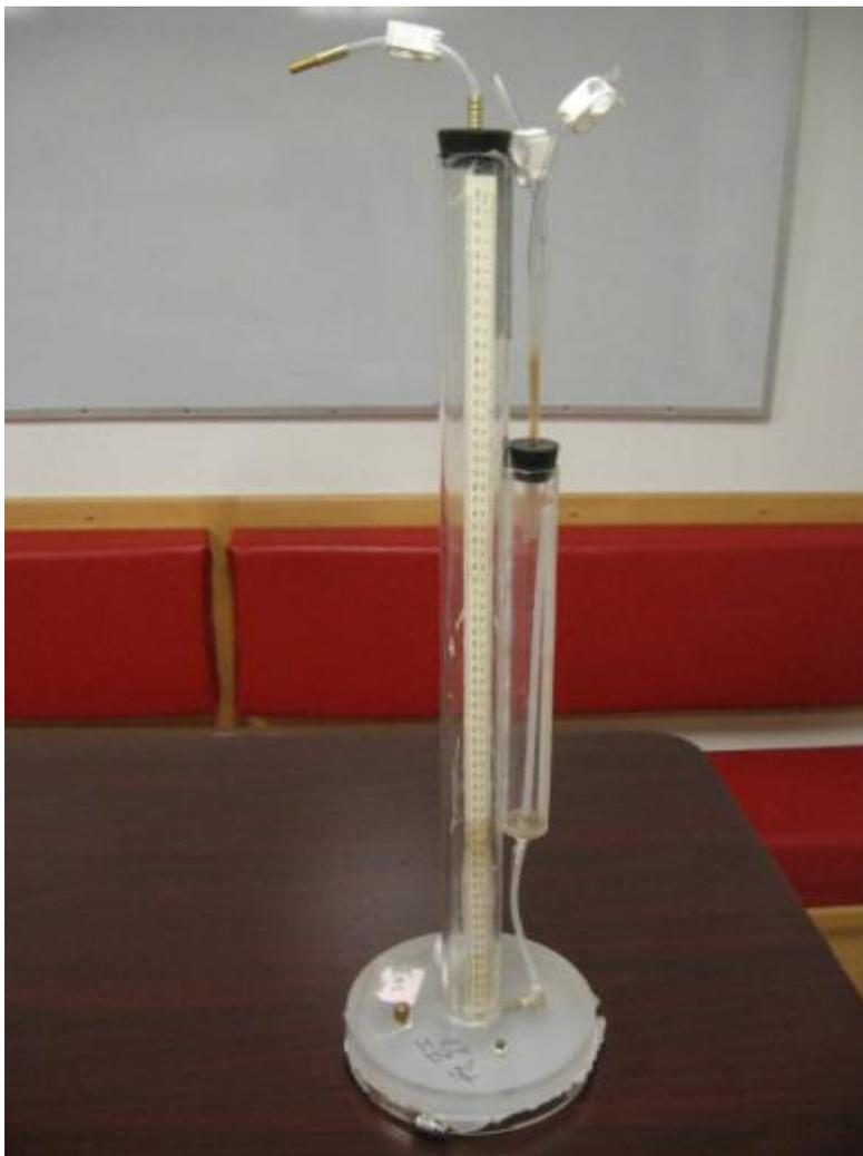
Figure 7. Tension Disk Infiltrometer test kit.
