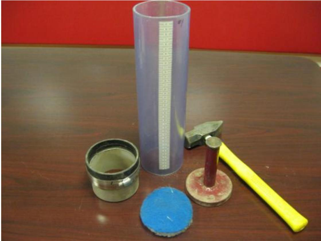
Figure 5. MPD test kit.
