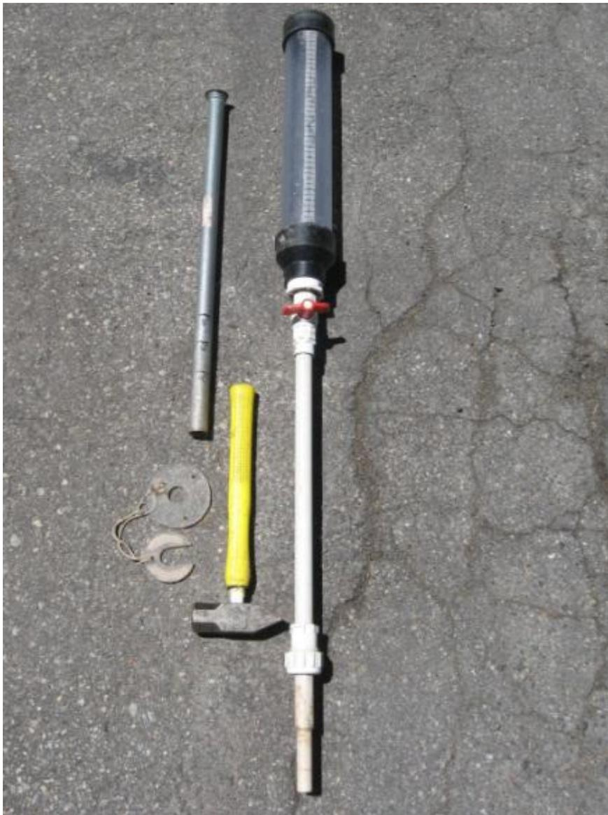
Figure 6. Constant Head Permeameter test kit.
