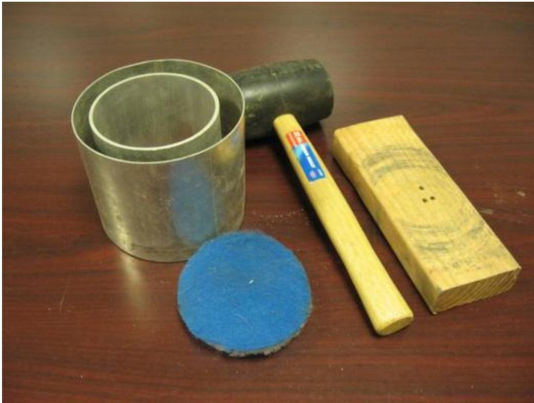
Figure 8. Double-ring infiltrometer test kit.
