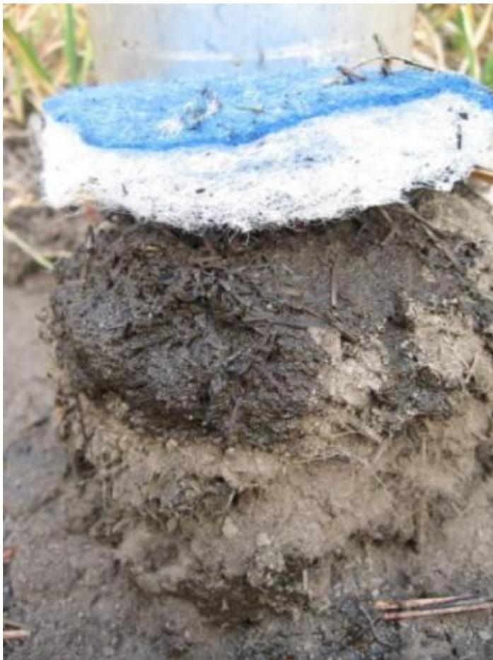
Figure 9. Hydrophobicity at the dry basin sample site. This DRI soil core had 3 inches constant head sustained for an hour.
